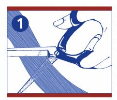
1. Cut the edgebanding 3 cm longer than surface to be covered. Make sure the surface is dust-free, clean, and dry. Also check to see there are no rough spots on the surface.
