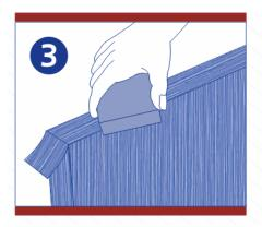
3. While still hot, press firmly with a wood block to the board.
