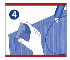
4. Allow the edgebanding to cool completely, remove the extra edges with a trimmer or a cutting blade and sand the edges.
