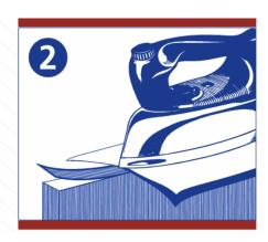
2. Apply the edgebanding with hot iron or hot air blower as described. It is recommended to use paper to protect iron bottom.
